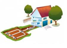
Geoexchange works on the principle that within a few feet of the surface, the earth remains a nearly constant temperature year round. In winter the ground is slightly warmer, and in summer slightly cooler than the air. Geoexchange simply moves and compresses the low grade temperature difference (heat or
