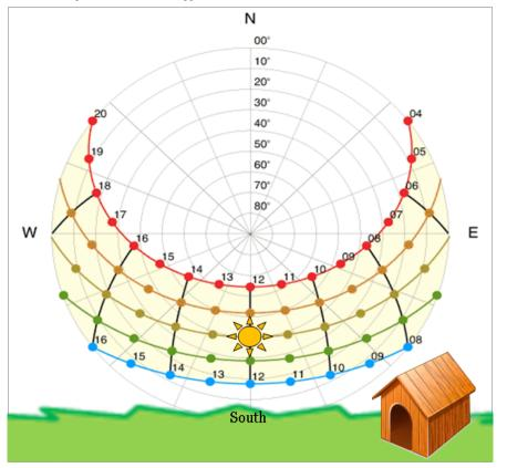
These diagrams can be used to estimate shading for a particular location throughout the year.
