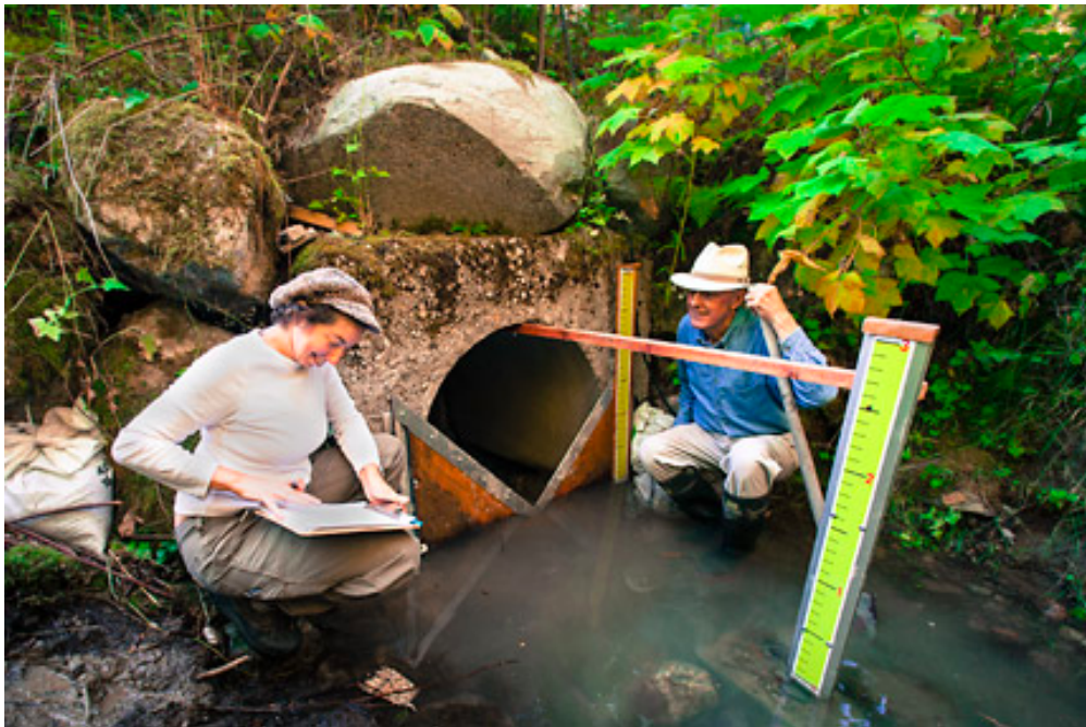
Swami Sivananda and a Karma Yogi monitoring the stream flow weir installed in Krishna Creek to assess how much power a mini-micro hydro generator could produce.
